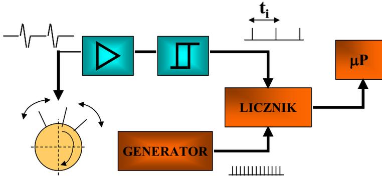
Fig.5. Structure of measurement tract used by diagnostic system SNDE-1b/SPL-2
